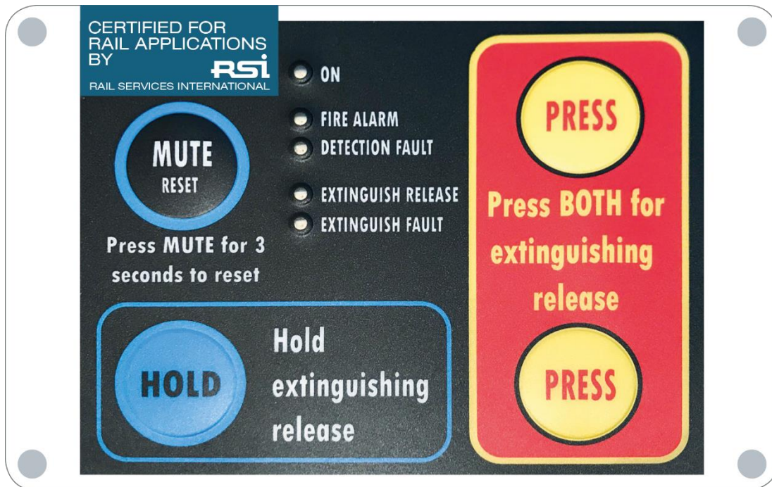
Figure 3 - SFCP Rail front panel controls and indications
